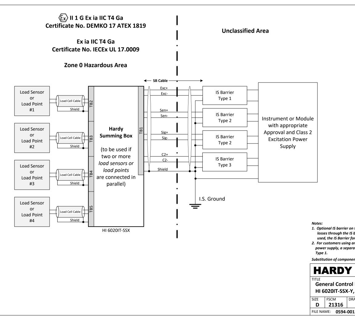
Optional IS barrier on the sense lines is used to automatically compensate for losses through the IS barrier on the excitation lines. If the sense lines are not used, the IS Barrier for the sense lines is not required
