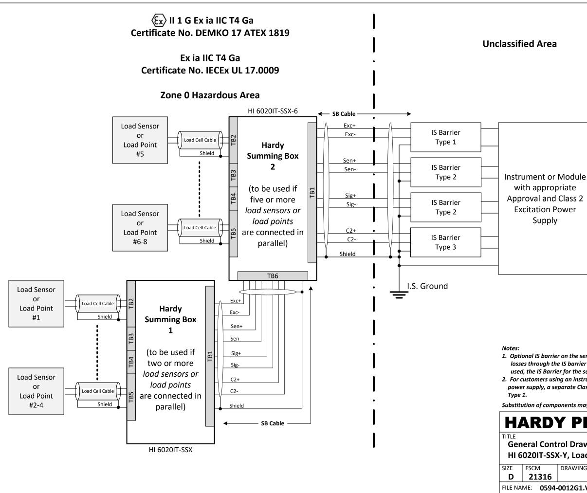
1. Optional IS barrier on the sense lines is used to automatically compensate for losses through the IS barrier on the excitation lines. If the sense lines are not used, the IS Barrier for the sense lines is not required 2. For customers using an instrument or module without a Class 2 rated excitation power supply, a separate Class 2 power supply can be used to power IS Barrier
